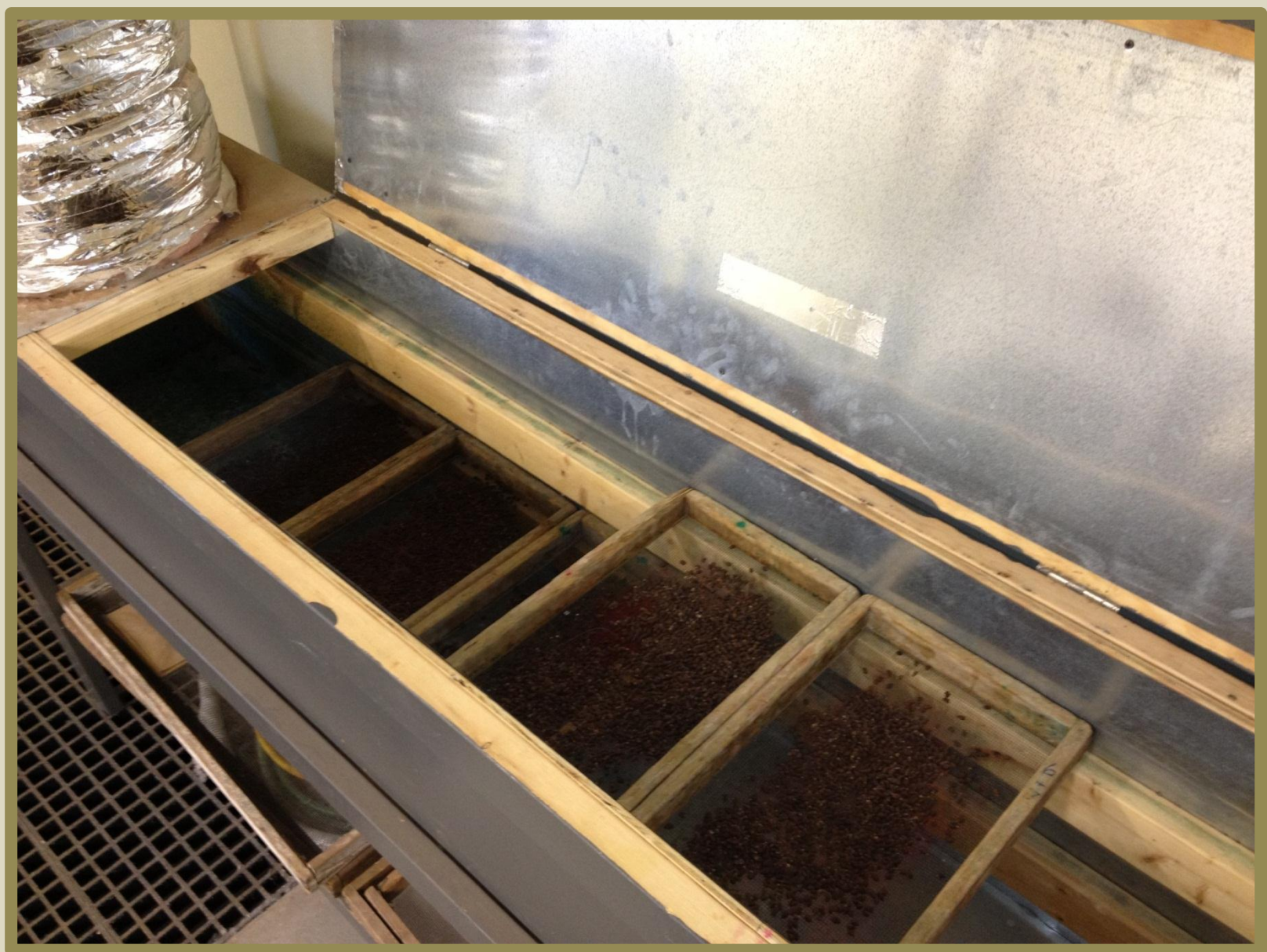
Dryer Box- The box was built using 2x4 inch lumber and 1/4 inch plywood with a sheet metal lining to help hold in the heat. With dual levels this box allows a maximum of 30 racks to be dried simultaneously. The entire top opens for easy access and to allow for cleaning.
