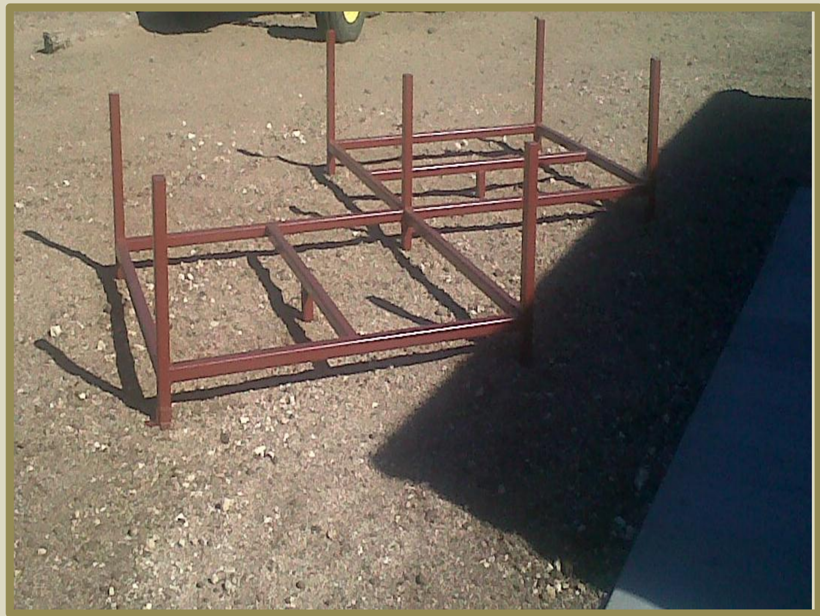
Tank Rack- 2x2x1/8 inch square tubing elevates tanks off ground level to prevent wear and hold tanks in place.
