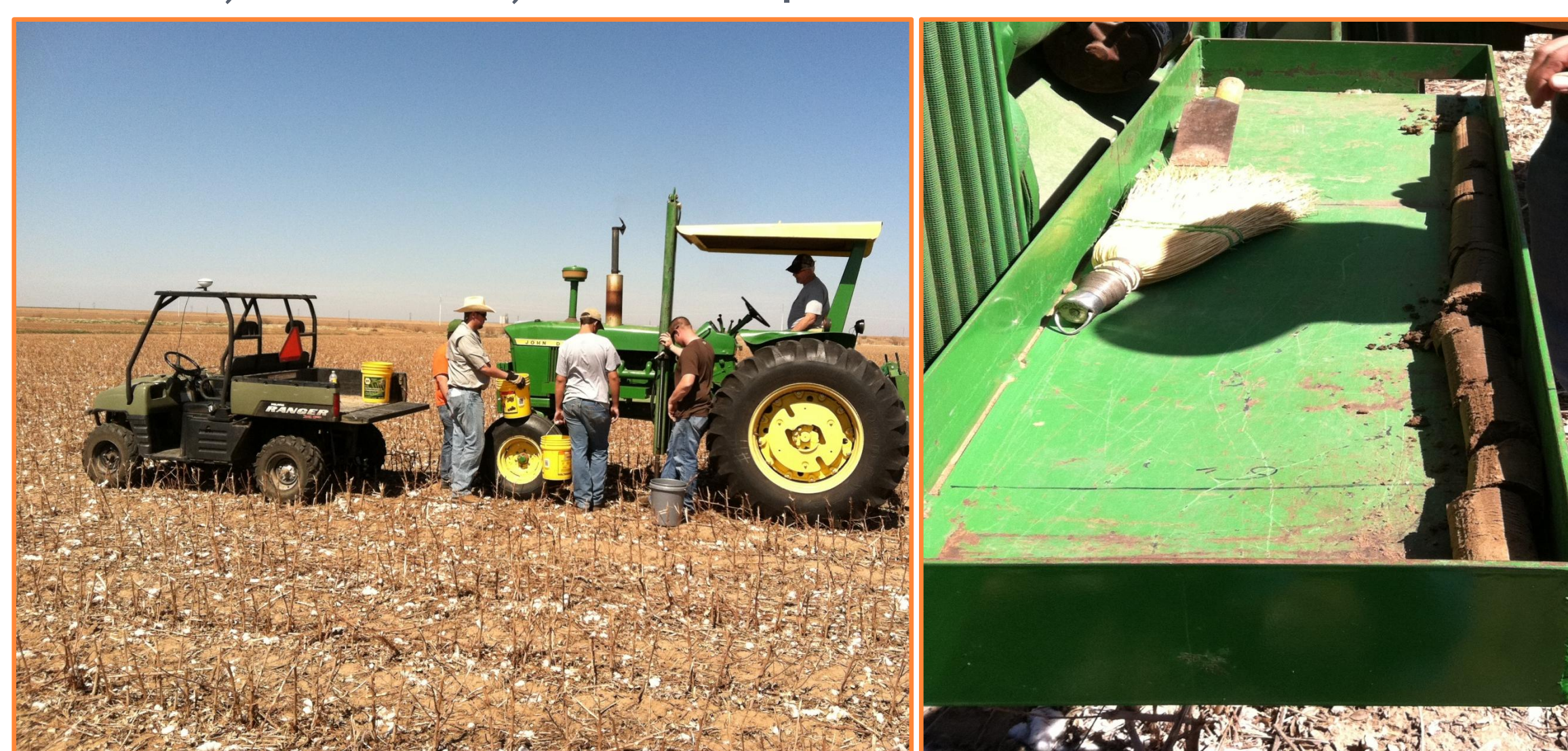
Figure 3. Soil sampling method: On the left is a tractor with a hydraulic soil probe and on the right is a tray where soil cores were divided into respective sub-samples.
