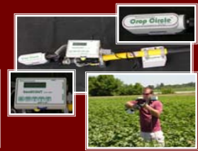
Fig. 10. Crop Circle unit model ACS-210 and data collection; an active sensor emitting 880 ± 10 nm and 650 nm.
