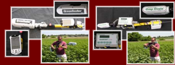
Fig. 9. GreenSeeker unit model 505 and data collection; an active sensor emitting 770 ± 15nm and 650 ± 10nm.
