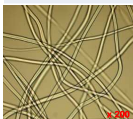
Fibres of G. hirsutum after NaOH treatment
